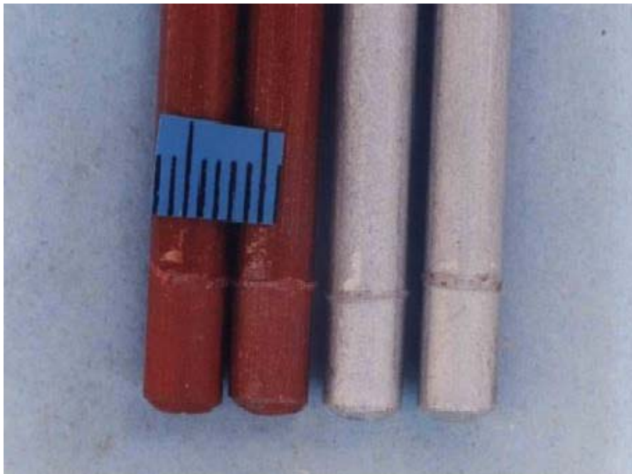
Figure 4: Tip of rutile underwater wet welding electrodes with double waterproof coating (1)
