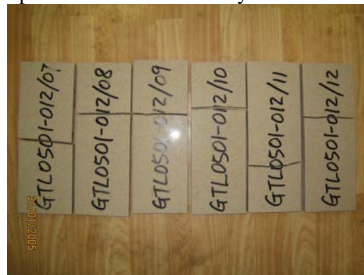
Specimens tested under dry condition
